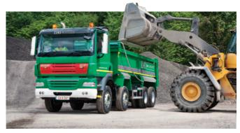
features required by Crossrail include a side scan system and side guards to protect cyclists and other road users. A reversing camera and white noise bleeper, twin hazard beacons, front and rear strobe lights, and wheelnut indicators were also specified for these tippers.
